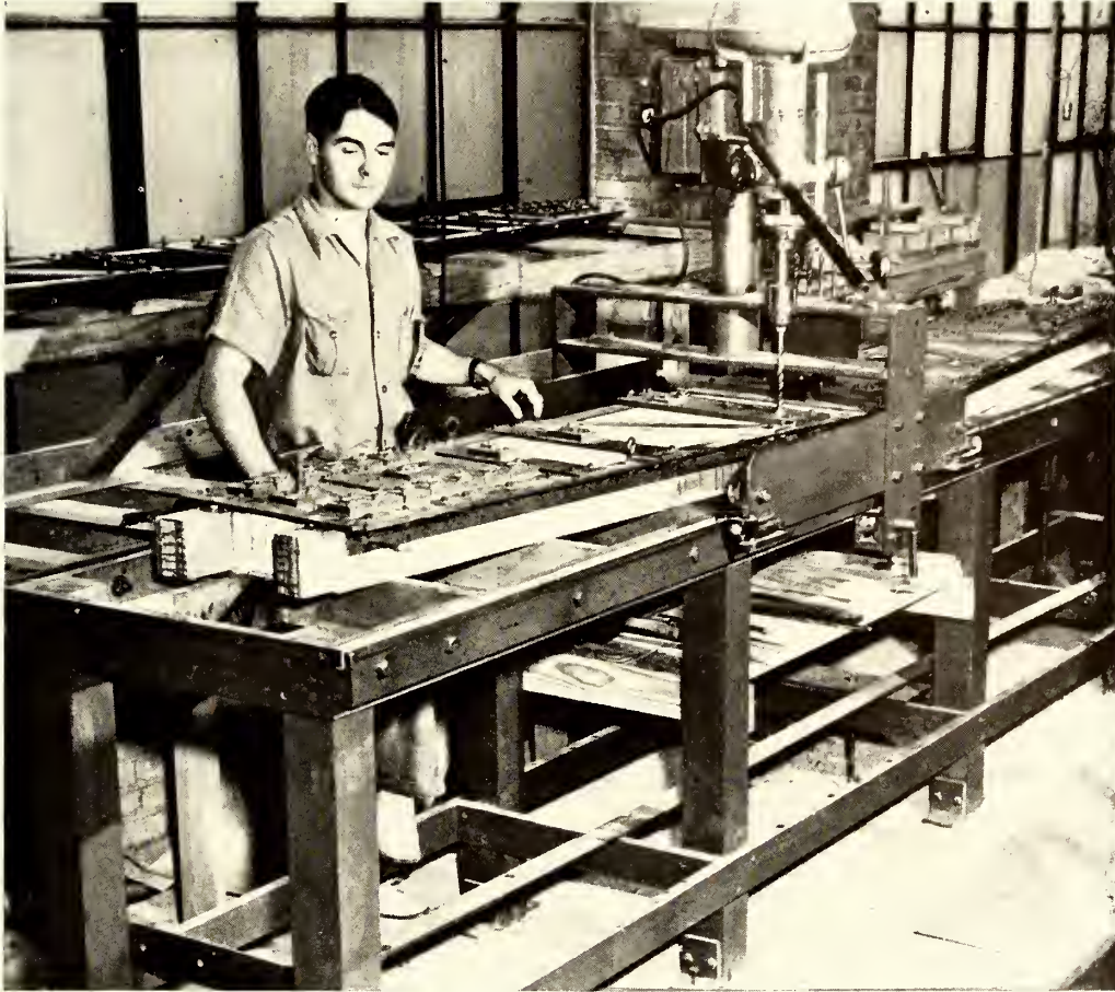
FIGURE 5-87.—Template for boring spar shear webs.
